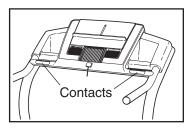
your heart rate accurately. Before using the handgrip pulse sensor, remove the clear plastic film from the metal contacts. In addition, make sure that your hands are clean.
